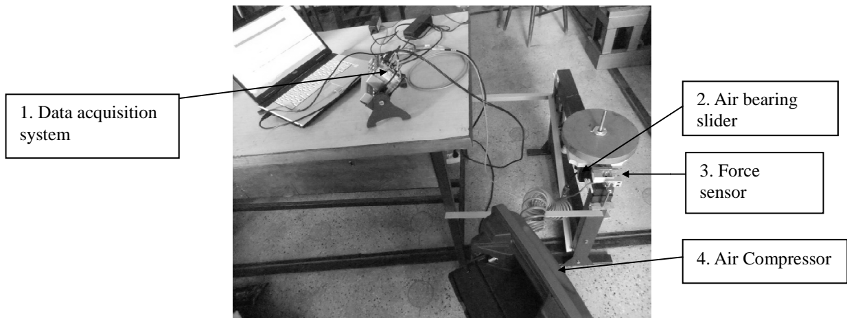
Figure 2 Experimental arrangement for the measurement of centrifugal force
